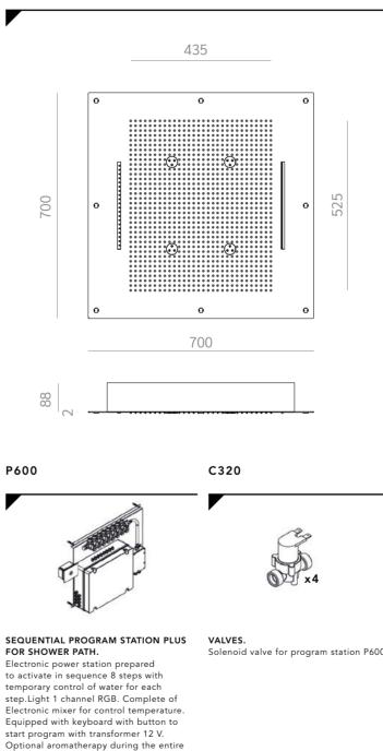
. program. N.B. To be teamed with a single wiring electrovalve C320 12V for each step.
